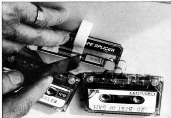
Surplus splicing tape is trimmed with a sharp knife
